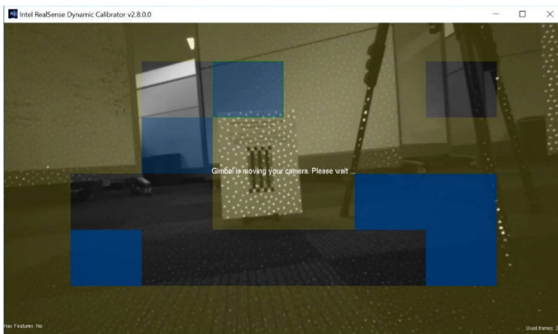
Figure 5-3 Hybrid Dynamic Calibration – Target-less Phase
