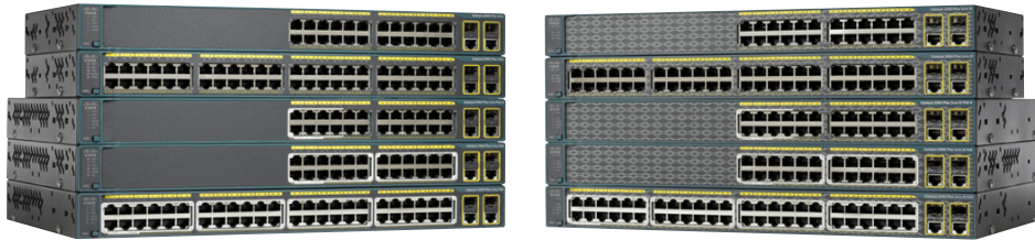
Figure 1. Cisco Catalyst 2960-Plus Series Switches
